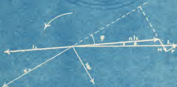
Fig. 2. Vector Diagram of Current Transformer on Inductive Load.
